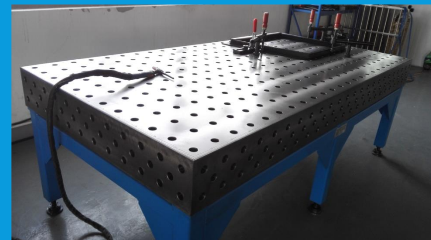
三维焊接平台及夹具 ( 3D welding work platform )
